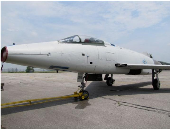
Painting of 081 has begun. The vertical tail has been painted with the required 3 color camouflage (dark green, medium green and tan) and the bottom of the fuselage has been painted light gray.
