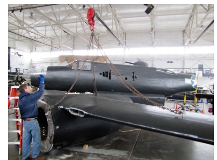
Left Wing ready for installation
