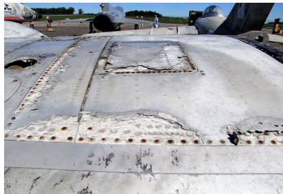
Left Wing Corrosion
