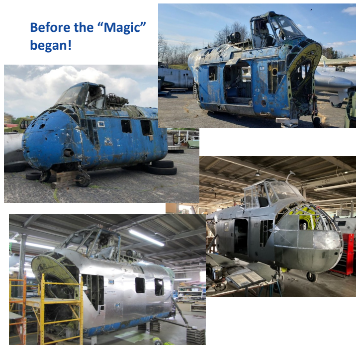
Most of the helicopter's outer skin needed replacing and much of it has been fabricated and installed pending final riveting.
