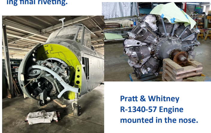
Most of the helicopter's outer skin needed replacing and much of it has been fabricated and installed pending final riveting.
