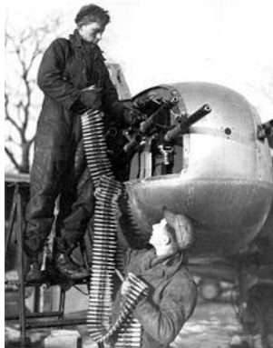
Re-loading machine guns on an A-26B with a six-gun nose The large majority of the A-26/B-26 Invader's production run of 2,452 were early A-26Bs and A-26Cs.
