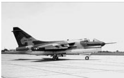
YA-7D-1-CV AF Serial No. 67-14582, the first USAF YA-7D, 2 May 1968. Note the Navy-style refueling probe and the modified Navy Bureau Number used as its USAF tail number.
