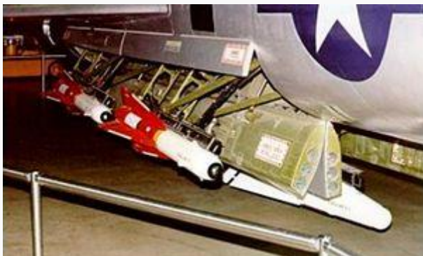
A pair of AIM-4D Falcons in the weapons bay of the F-102 Delta Dagger fighter
