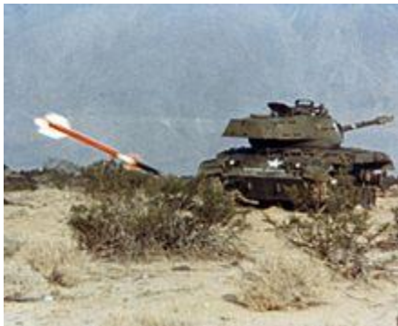
Experimental use of an AIM-9L against tanks at China Lake, 1971.
