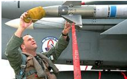
AIM-9M Sidewinder with distinctive "Dash-9" lettering being pre-flighted by a USAF pilot. Note the blue stripe, which indicates that this example has an inert warhead intended for training purposes
