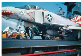
An F-4B of VF-111 on the USS Coral Sea armed with AIM-9Ds
