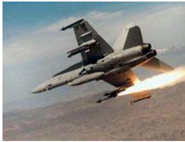
AIM-9R test firing from an F/A-18C at Naval Air Weapons Station China Lake
