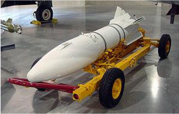
AIR-2A Genie nuclear air-to-air rocket on a MF-9 Transport Trailer at Hill Aerospace Museum
