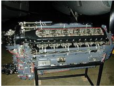
Cutaway of Allison V-1710
