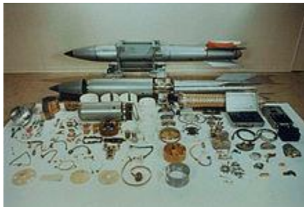
B61 bomb in various stages of assembly. The nuclear component is contained in the small, silver cylinder near the upper middle.
