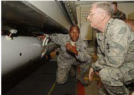
Inert training version of a B61 in an underground Weapons Storage and Security System (WS3) vault at Volkel Air Base, Holland. An access panel on the warhead is open, showing the interface for actions such as PAL (safety/arming) and variable yield setting.
