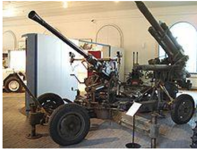
Finnish Bofors 40 mm. This gun mounts the original reflector sights, and lacks the armor found on British examples.
