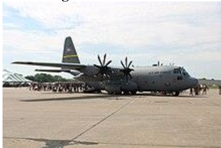
C-130H with eight-bladed NP2000 propellers
