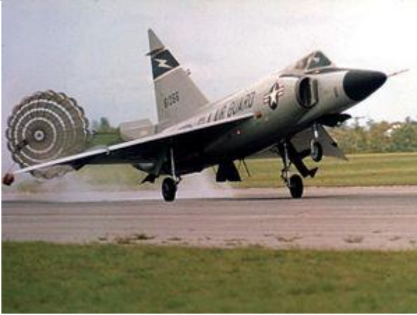
F-102 from the 125th Fighter Interceptor Group, Florida Air National Guard, deploys braking parachute
