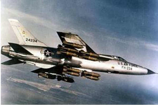
A Republic F-105D-30-RE Thunderchief in flight with a full bomb load of sixteen 750 lb bombs on its five hard points.
