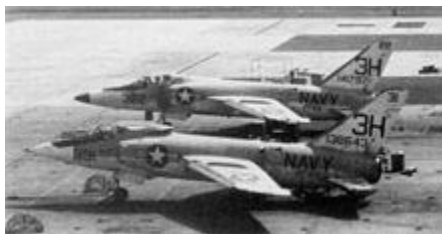
An early production "short nose" F11F and a later "long nose" from VT-23.
