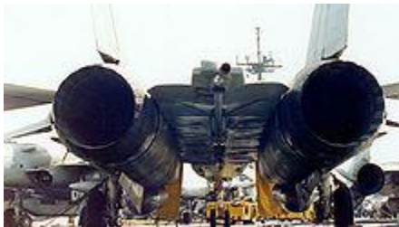
F-14's large flat area between the engine nacelles is called the "pancake".
