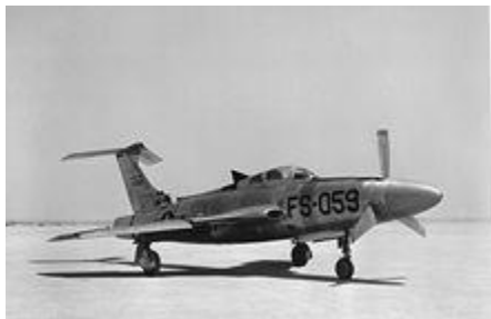
The Republic XF-84H Thunderscreech prototype.
