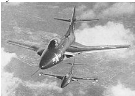
A swept-wing F9F-6 Cougar (foreground) and a straight-wing F9F-5 Panther in flight
