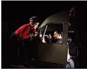
Riveting team working on the cockpit shell of a C-47 transport at the plant of North American Aviation. Office of War Information photo by Alfred T. Palmer, 1942.
