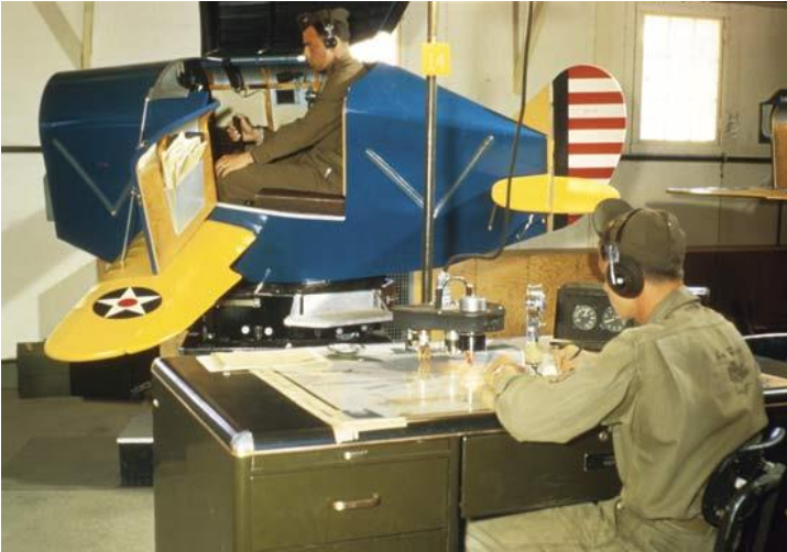
Flight simulation in the C-3 Link Trainer, U.S. Army Air Forces, 1940s. A cadet takes the controls, and a nearby instructor relays commands by telephone.
