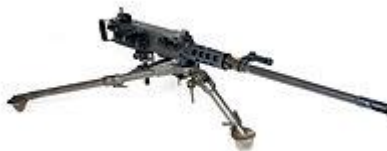
The M2E2 modification with quick-change barrel
