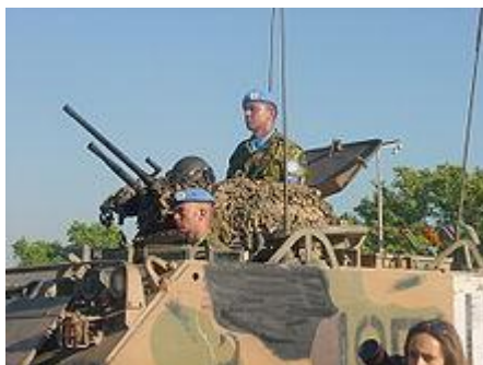
Australian M113 with twin mounted M1919 Browning and M2 Browning Quick Change Barrel machine guns.
