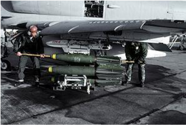
Crewmen upload three Mark 81 general purpose high explosive bombs, with Mark 14 TRD (Tail Retarding Device) attached, aboard an A-4F Skyhawk aircraft from Marine Attack Squadron 133 (VMA-133).
