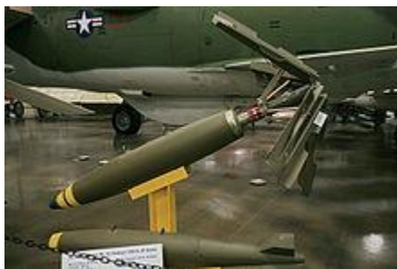
Mk. 82 bomb with Tail Retarding Device – this photograph shows an unfuzed, museum display Mk 82 with its usual combat paint scheme. For display purposes, the optional high-drag "Snakeye" tailfins used for low-altitude release are shown.
