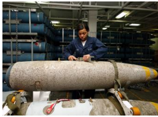
An aviation ordnance technician handling the bomb body of a Mark 84 aboard the USS George Washington .
