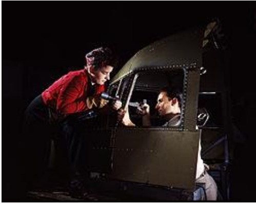
Man and woman riveting team working on the cockpit shell of a C-47 aircraft at the plant of North American Aviation (1942).
