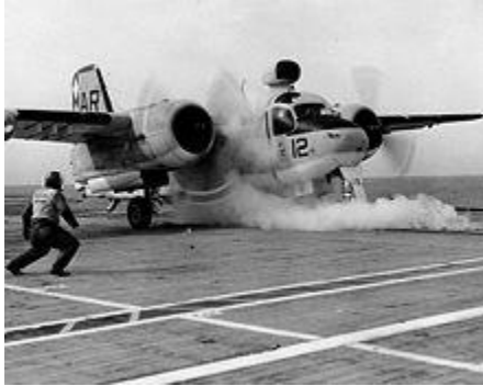
US Navy S-2 Tracker on the port catapult of USS Lexington (CVS-16) ready for take-off, 22 January 1963
