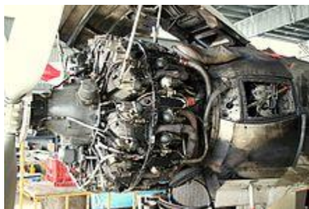
Wright R-3350 Turbo-Compound radial engine fitted at the Number Four position on the starboard wing of a Lockheed Super Constellation
