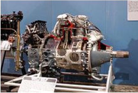
A Wright R-3350 radial engine, showing, R to L, propeller shaft, reduction gear case, magneto (silver) with wiring, two cylinders (rear with connecting rod), impellor casing (and induction pipe outlets) and injection carburetor (black); separate accessory gearbox at extreme left..
